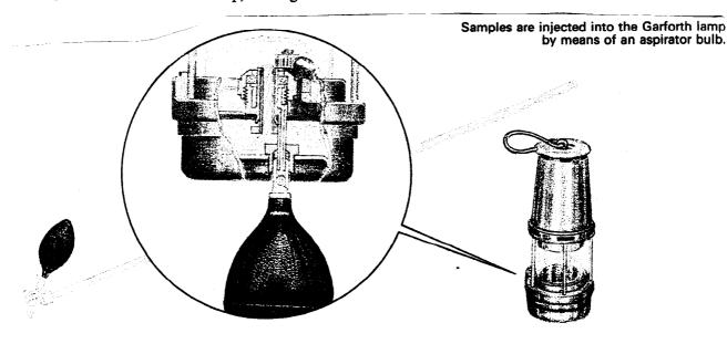
If the point to be sampled is not within arm's reach, the sampling bulb needs to be fitted to a special sampling valve and held at the end of a rod. The valve lever is depressed when deflating or inflating the bulb.
